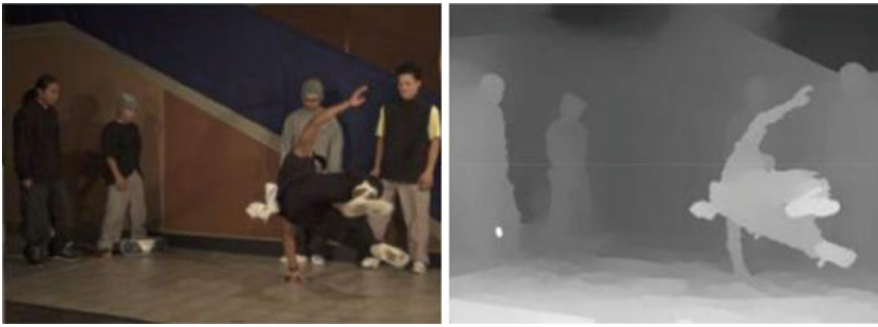
Fig. 2.8 Sequence breakdance: video ( left ) plus depth ( right )
