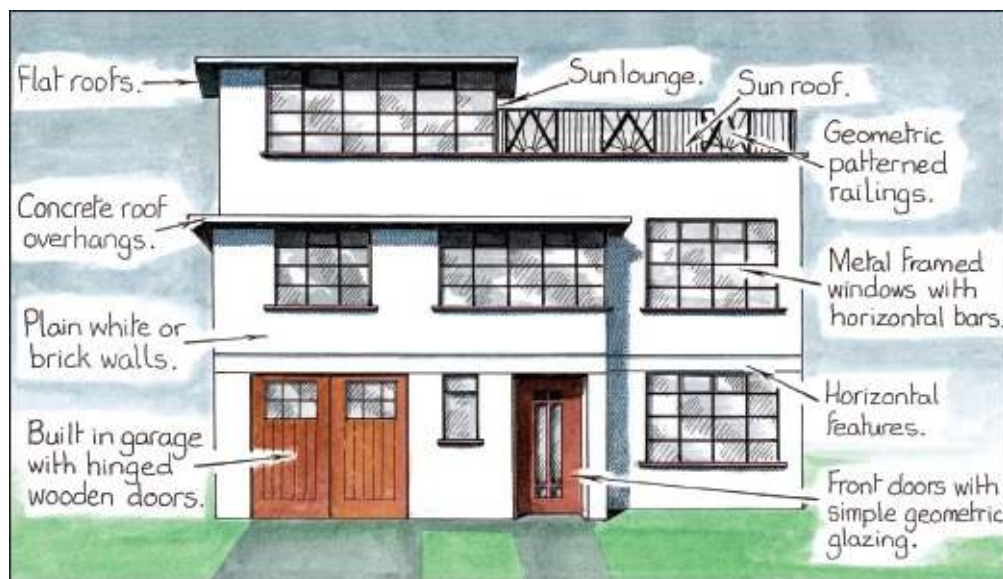
FIG 2.3: An International Style house with labels of its distinctive features. This British version of Modernism (also referred to as the Horizontal Style or Ultra Modern) was named after an exhibition titled 'The International Style' held at the Museum of Modern Art, New York in 1932.
