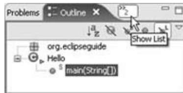
Figure 2-3. Views can be stacked on top of one another. If space is short, some may be hidden in a chevron menu.
