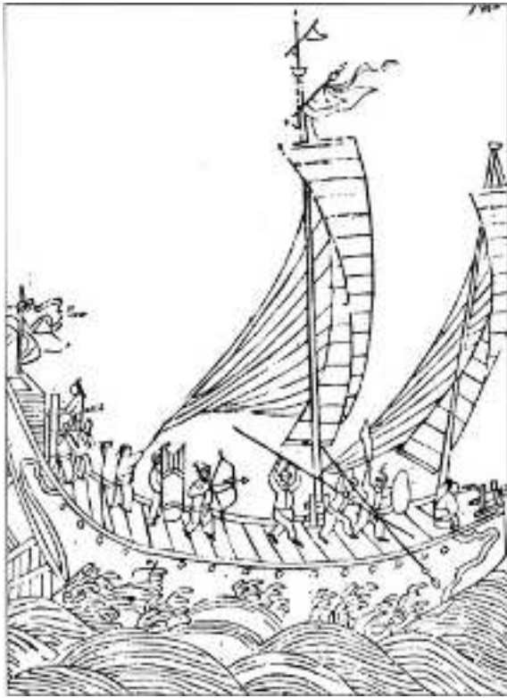
A smaller warship of Jiangsu style depicted in the Wu Bei Zhi of 1628. The vessel carries a small cannon in its bow.
