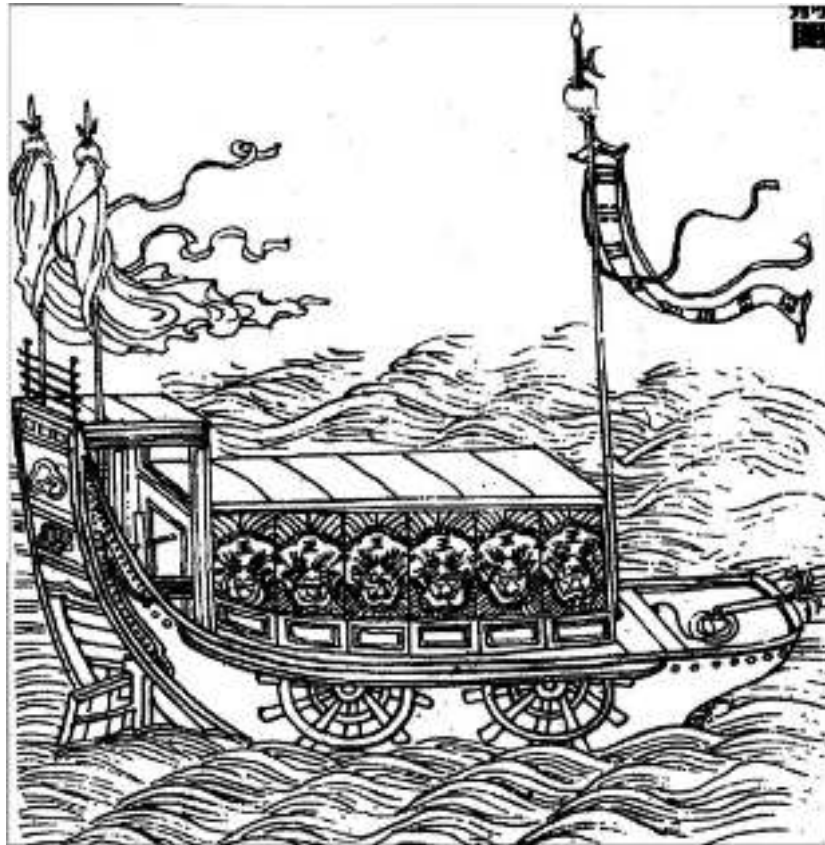
A four-wheeled paddle-wheel warship, with tigers' faces painted on to the sides, which could be let down for boarding.
