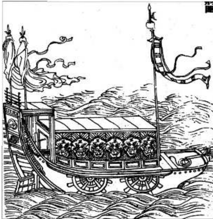
A four-wheeled paddle-wheel warship, with tigers' faces painted on to the sides, which could be let down for boarding.
