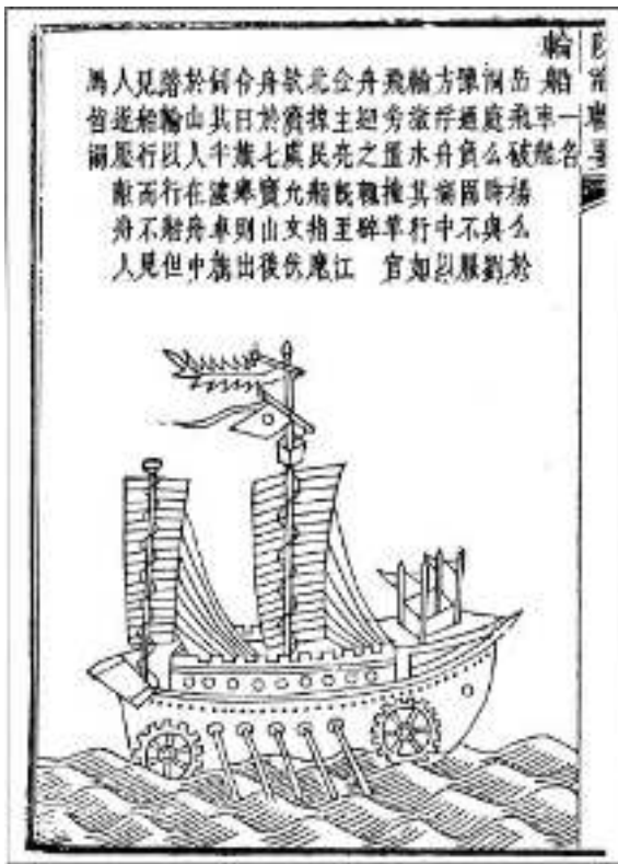
A charming drawing of a Chinese paddle-wheel warship of the Song dynasty which appeared in an 1842 edition of a work on coastal defence.
