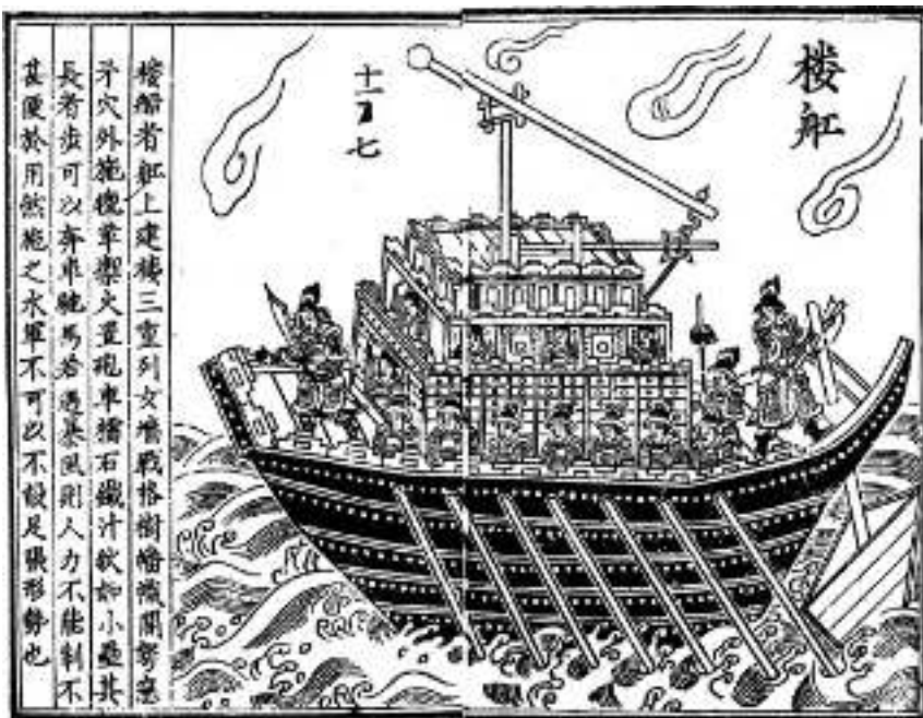
The lou chuan (battleship) in the 1520 edition of Wu Jing Zong Yao (AD 1044). It has the characteristic open construction whereby the oarsmen are protected only by the ship's gunwales. Its offensive armament is a counterweight trebuchet.
