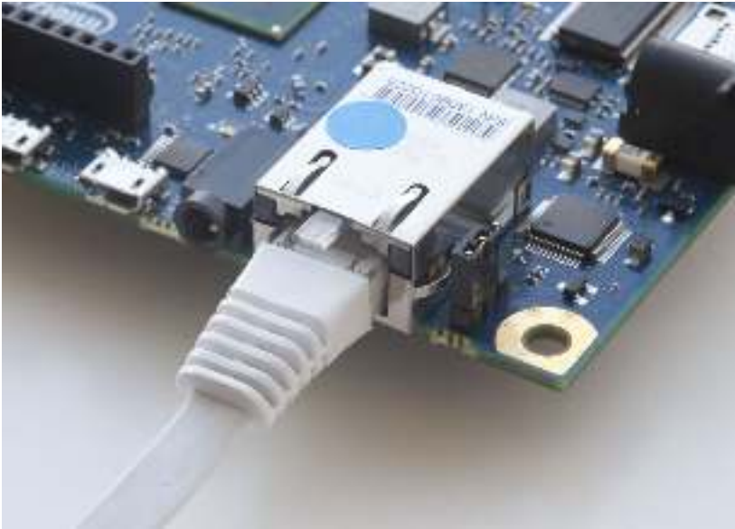
Figure 1-3. The Galileo's Ethernet port is just one way it can communicate with users or other devices.
