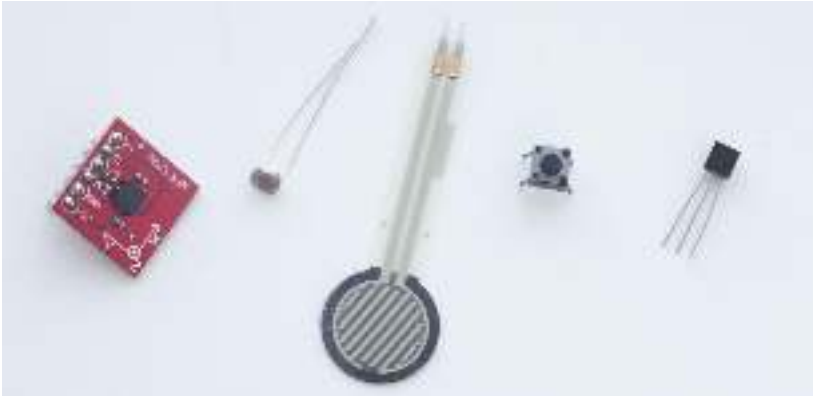
Figure 1-1. A few possible inputs. From left to right: an accelerometer, a photo cell, a pressure sensor, a button, and a temperature sensor.
