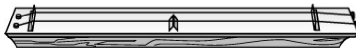
Fig. 2. The monochord with a stop halfway along the string. The full, unstopped string is also shown.
