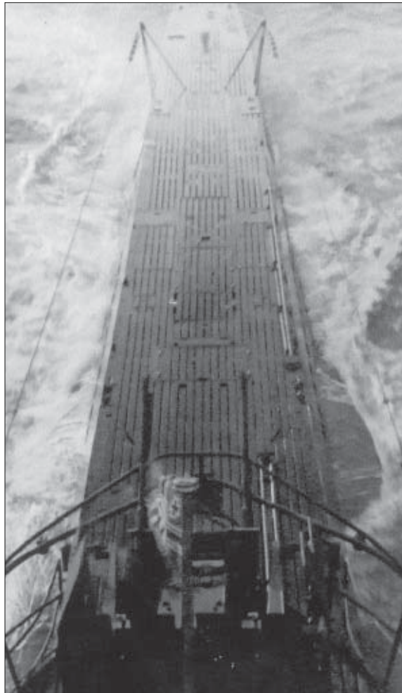
Looking towards the stern from the upper tower flak platform on a late-war Type VIIC. Clearly visible is the four-barrelled 2 cm Flakvierling , a weapon only fitted to a limited number of U-boats.
