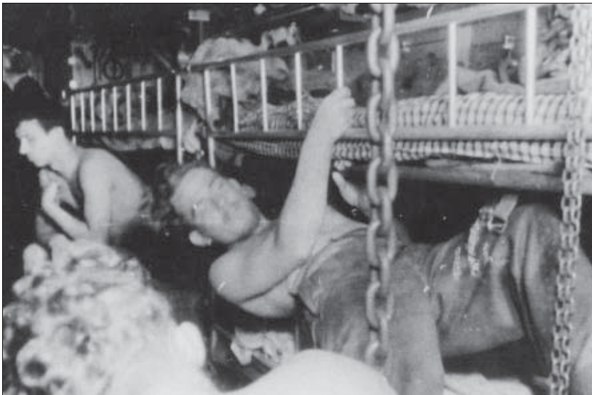
A view inside the bow compartment shows just how cramped living conditions were on an operational U-boat. The chains hanging down in the foreground are part of the torpedo hoist.
