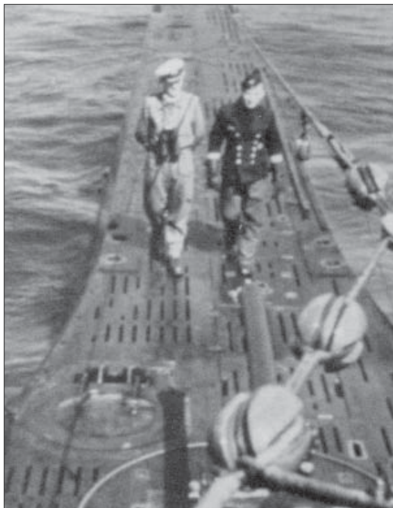
A U-boat commander and his L.I. (Leitender Ingenieur) stroll along the foredeck of their Type VIIC. The insulator blocks on the jump wires can be clearly seen. Note also the closed hatch for the ready-ammunition locker for the 8.8 cm deck gun just ahead of the commander.
