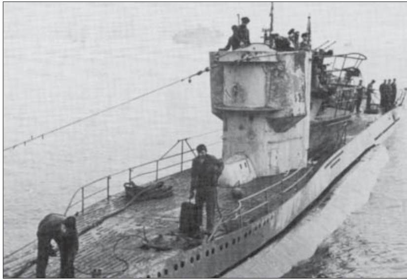
U-377, a Type VIIC, seen here after her bridge conversion. The armoured shelters, intended to give bridge crew some protection against enemy fire, can be seen welded to either side of the forward part of the tower. The deck gun has been removed and an extended 'wintergarten' platform fitted to the rear of the tower to take the upgraded flak armament. (Jak P. Mallmann-Showell)
