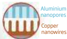
The nanowires and pores interlock, increasing contact area and creating the charge
