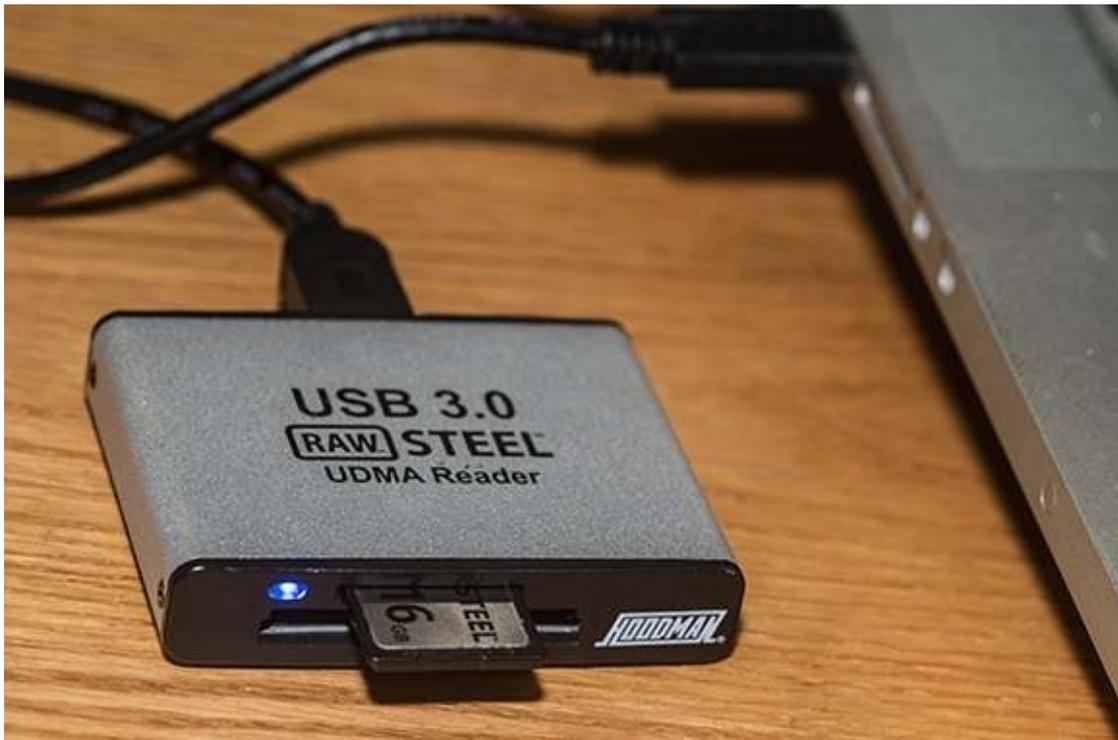
**QT.6** An SD memory card inserted into a Hoodman Raw Steel card reader, and connected to a laptop computer.
