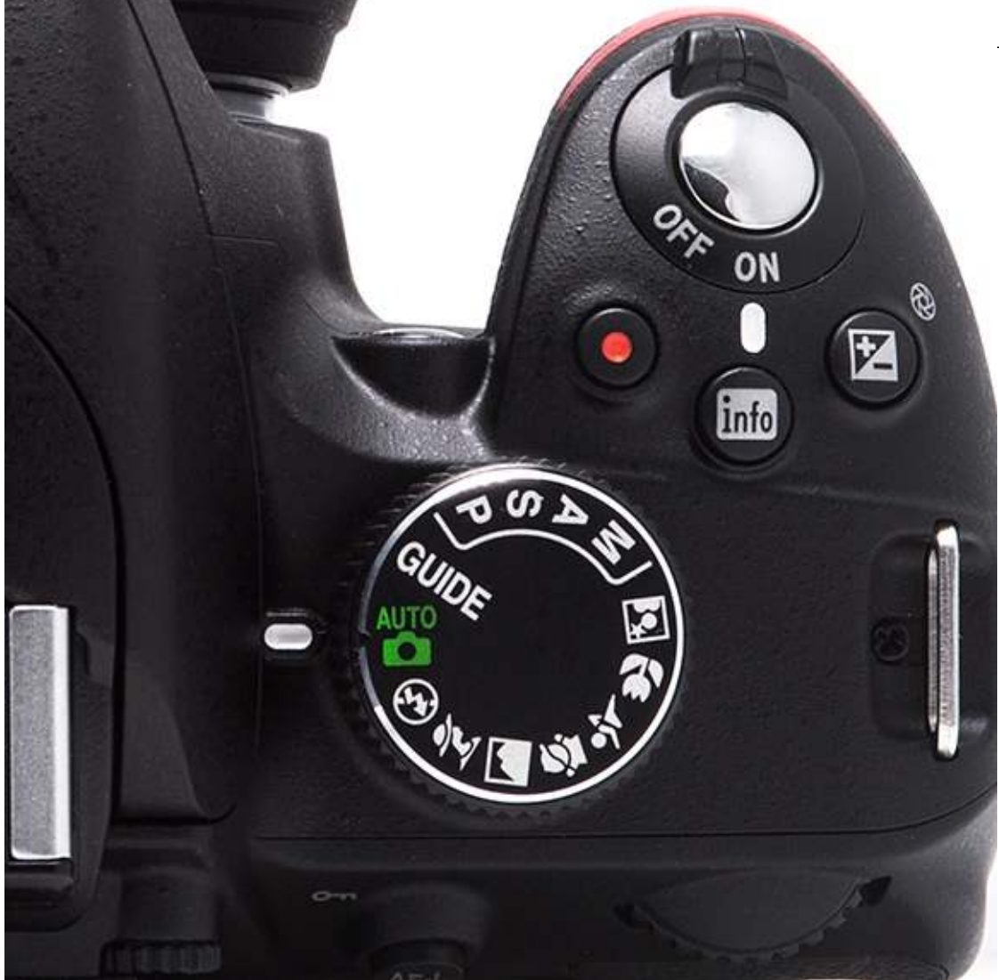
QT.2 The Mode dial showing the camera set to the Auto mode.
