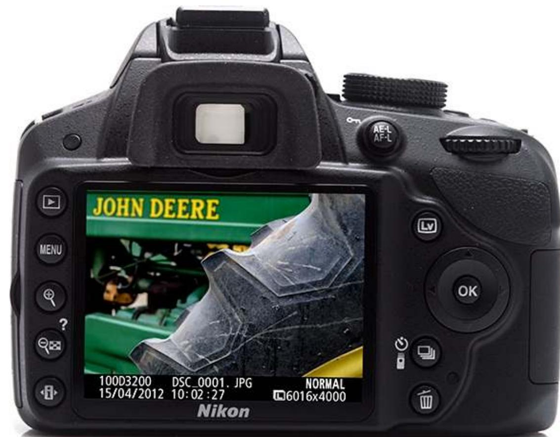
**QT.4** The back of the camera showing the last image taken with the photo data on the bottom.
