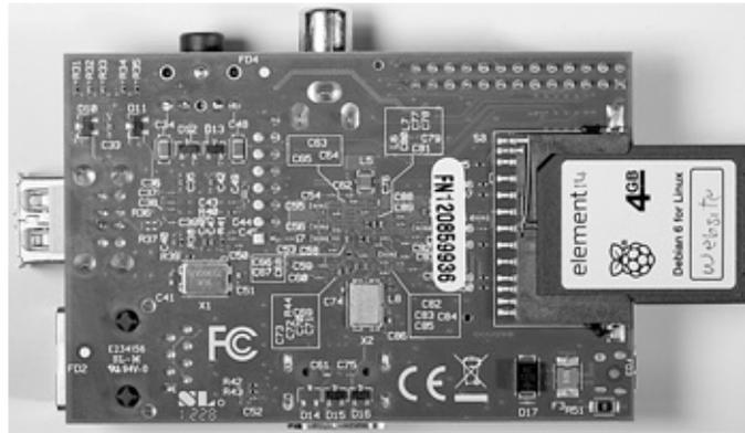
**Figure 1–3** Back side of the Raspberry Pi.
