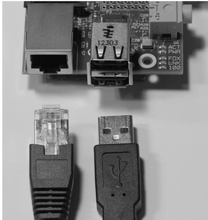
**Figure 1-12** Ethernet and USB connectors with cables.
