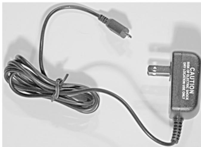
**Figure 1-6** External power supply.
