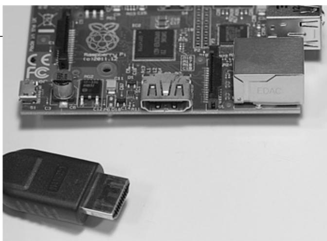
**Figure 1-7** HDMI connector and cable.
