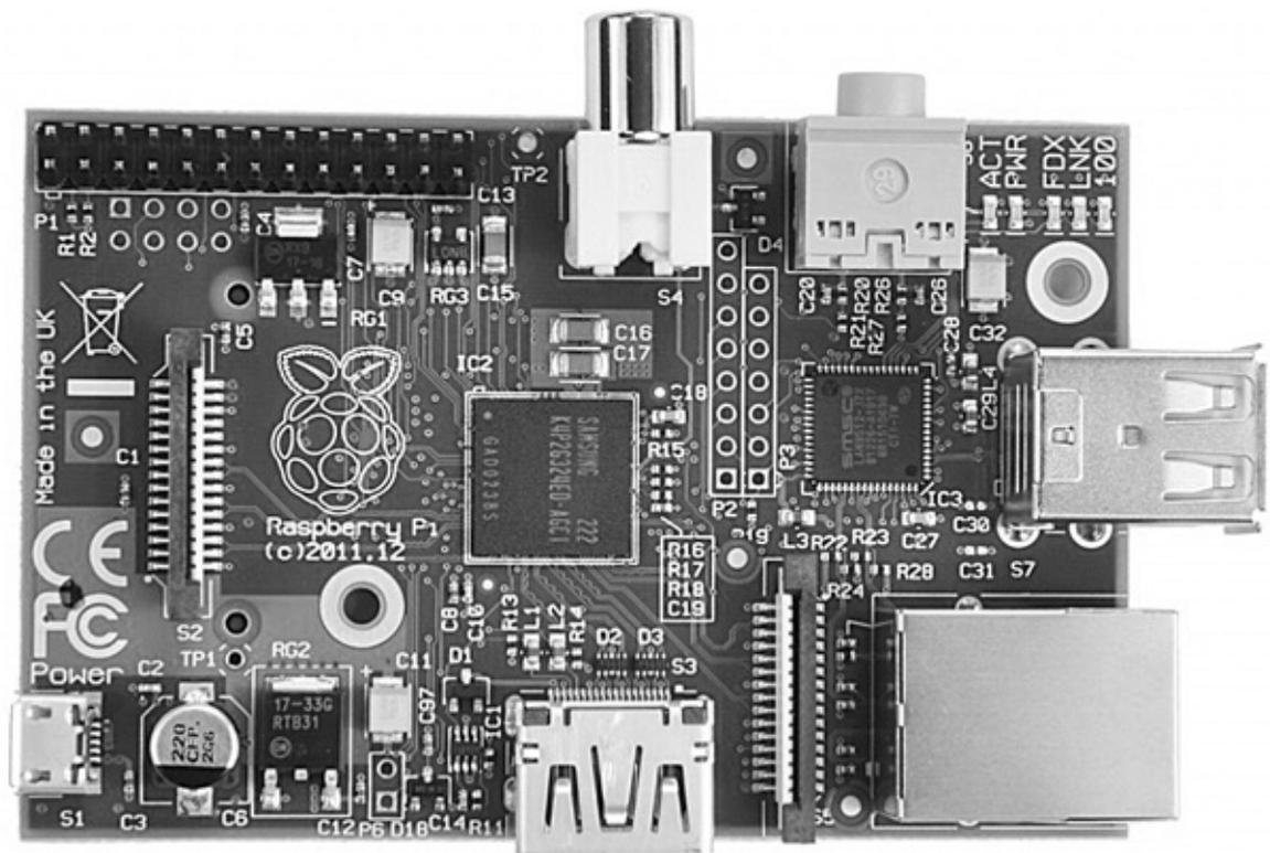
**Figure 1–1** The Raspberry Pi, a small Linux computer.
