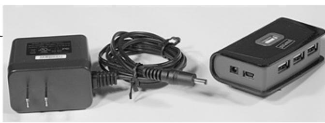
**Figure 1–13** Self-powered USB hub.
