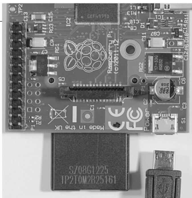
**Figure 1-5** Micro USB power connector.
