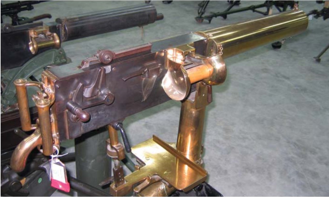
A transitional gun, combining Maxim's locking crank, fusee spring and belt-feed mechanism. Note the pistol grip and trigger. (Royal Armouries)
