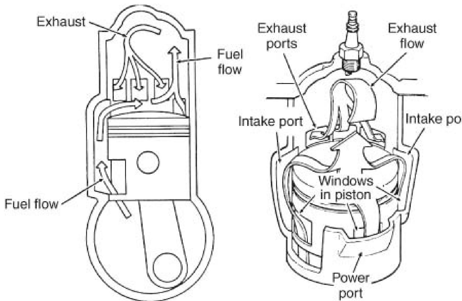
**Fig. 1-8.** *In a loop-scavenged engine the fuel charge enters through multiple transfer ports (called intake ports here) arranged around the periphery of the cylinder. Port exit angles to give swirl to the charge, which reduces short-circuiting. Windows in the piston skirt are an optional feature. OMC*
