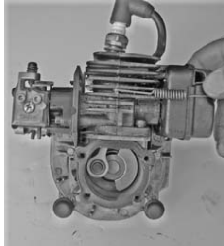
Fig. 1-6. Carburetors for third-port engines attach to the cylinder. Some of these engines incorporate a reed valve in the third port. Robert Shelby
