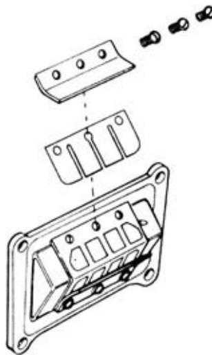
**Fig. 1-4.** *Multiple pedals are standard on high-performance engines. While there has been considerable experimentation with fiberglass, carbon fiber, and other high-tech materials, spring-steel pedals appear to work as well as any. Tecumseh Products Co.*
