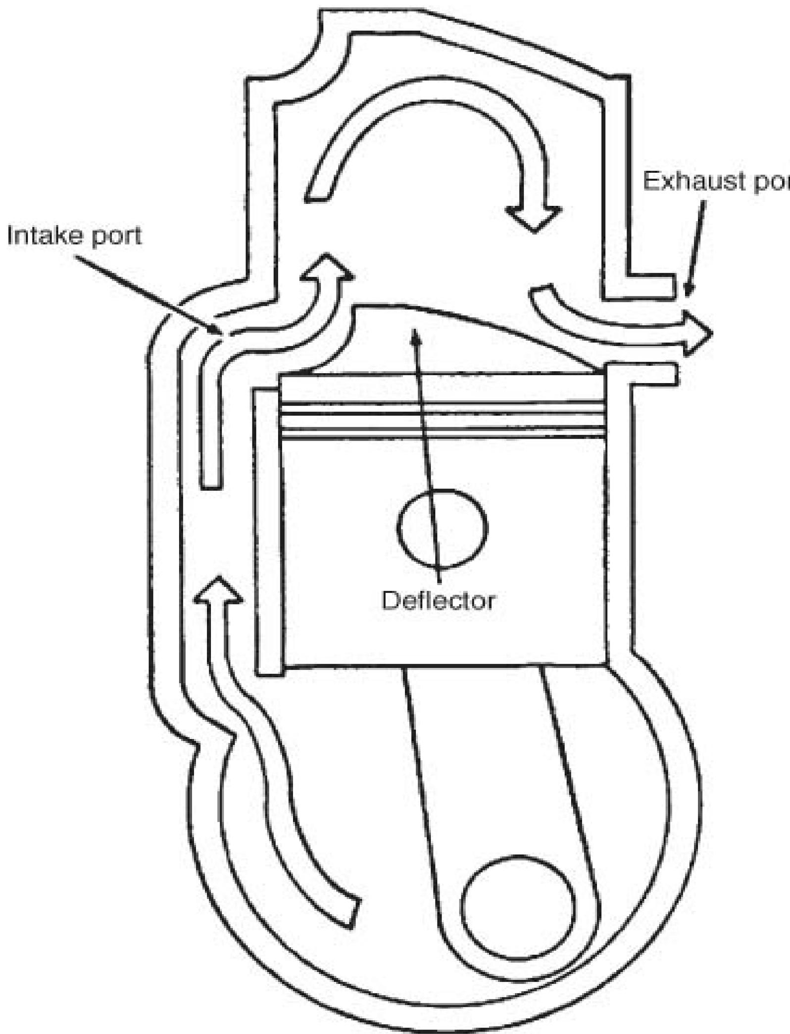
**Fig. 1-7.** *Cross-scavenged engines have the intake port 180° opposite the exhaust port. Incoming gas rebound upward off the deflector on the piston crown to give some protection against short-circuiting.*
