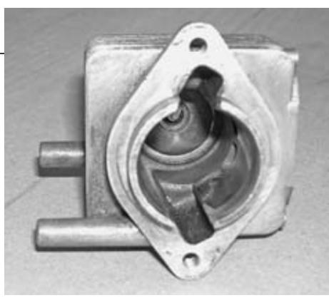
**Fig. 1-9.** This cylinder has what are sometimes called finger ports. That is, the transfer ports are open to the bore along their whole length. Looking carefully one can see the angled exit ramp at the upper end of lower port. Robert Shelby
