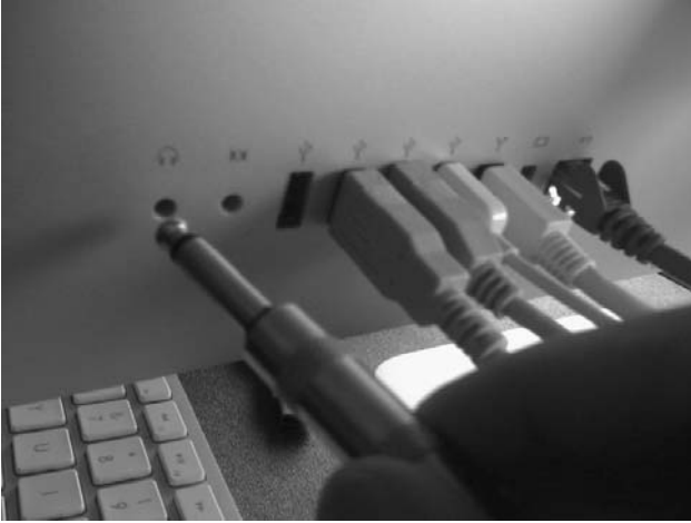
Figure 1.1 If you try to plug a guitar cord (1/4-inch) into this input, it won't fit.
